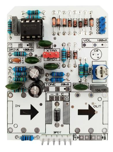
Solder the capacitors and transistors. If you have troubles reading the values, check out our <u>"Reading Part Values</u>" tutorial. Pay attention to the orientation, as well as to the polarity for electrolytic capacitors.
