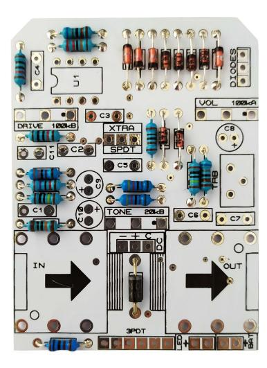
Place the resistors and diodes. If you have troubles reading the values, check out our <u>"Reading Part Values"</u> tutorial.
